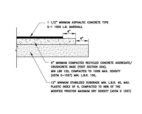
ASPHALT PAVEMENT SECTION W / CRUSHCRETE
